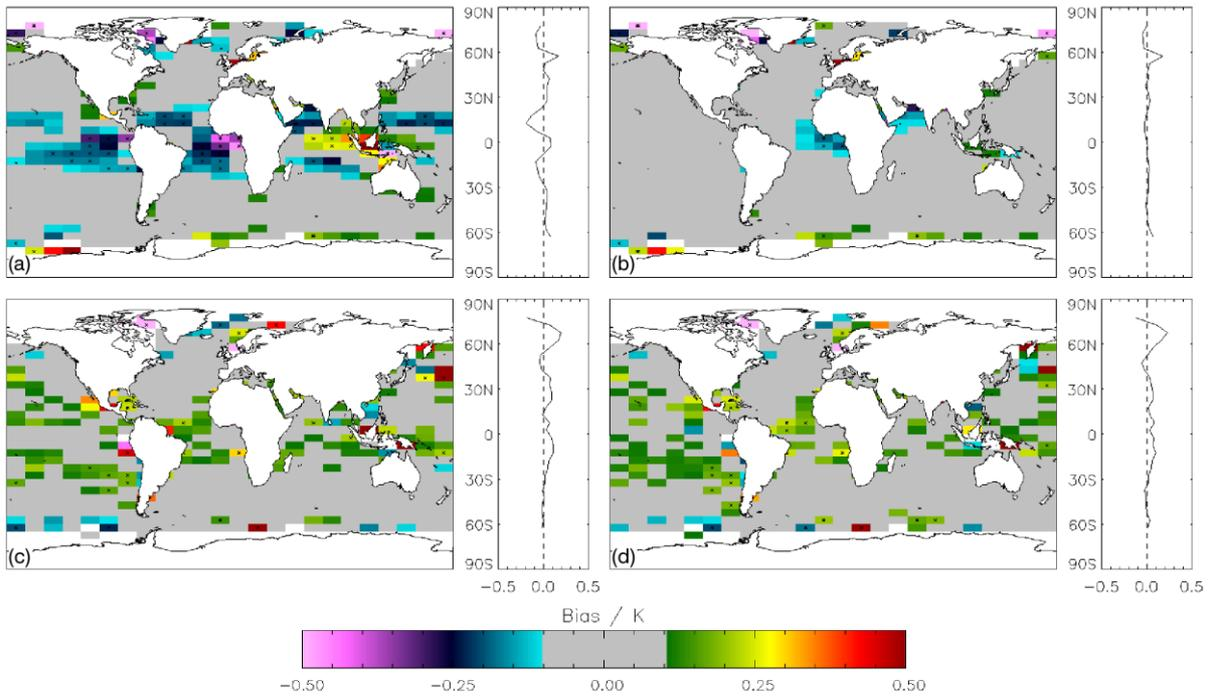
**Figure 1** Median difference between estimated  $SST_{0.2m}$  and in situ drifters for (a) AATSR D2, (b) AATSR D3, (c) ATSR-2 D2, and (d) ATSR-2 D3. X symbols indicate the difference exceeds 0.1 K with a significance of 90%, \* symbols indicate the bias exceeds 0.1 K with a significance of 99%. Significance is calculated with a Student's t-test using the number of unique drifters in each cell.
