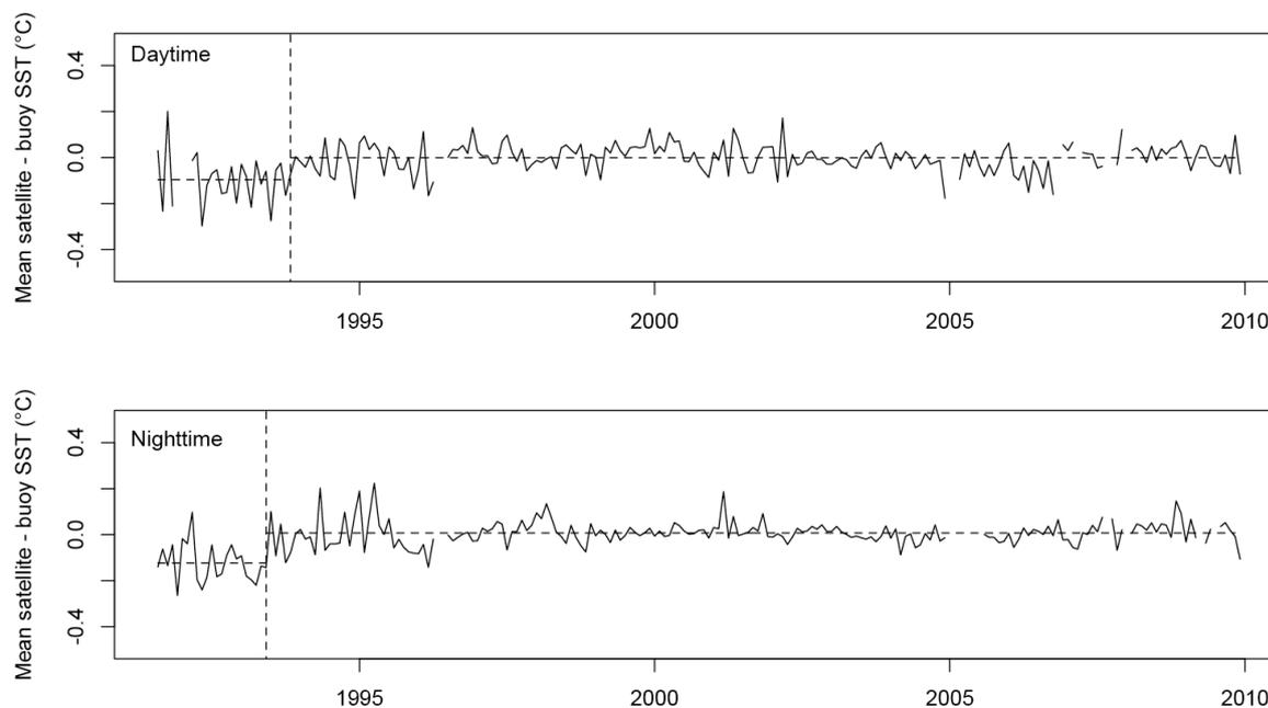
**Figure 3. Analysis of stability of the full series of ARC observations against tropical moored buoys, using a technique for identifying step changes objectively. Upper panel: daytime monthly mean discrepancies; lower panel, night time. The early step change is apparently associated with the dissipation of the post-Pinatubo stratospheric aerosol.**
